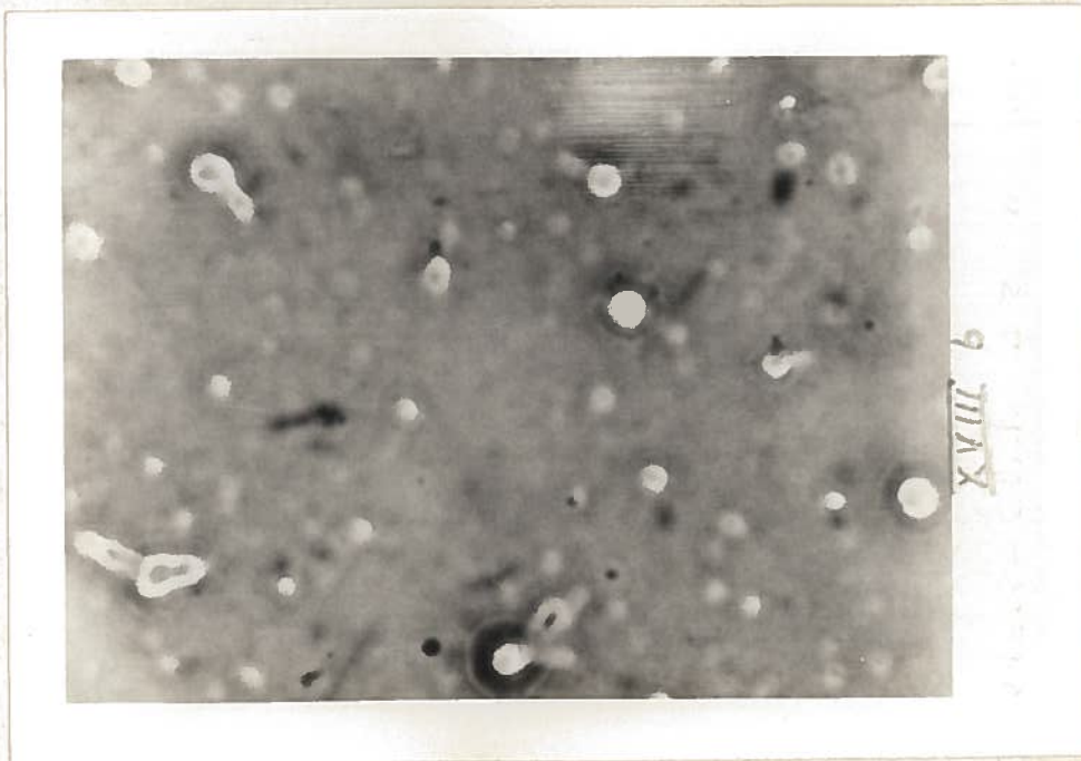
Figure XVIII(b). Photograph of Cellulose Acetate Butyrate Film Exposed to a Fast Neutron Flux. Bottom Plate
