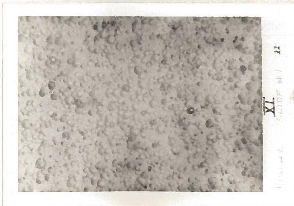
Figure XI. Photograph of Cellulose Nitrate Film Exposed to a Fast Neutron Flux for Use as a Basis for Flux Reduction Determination
