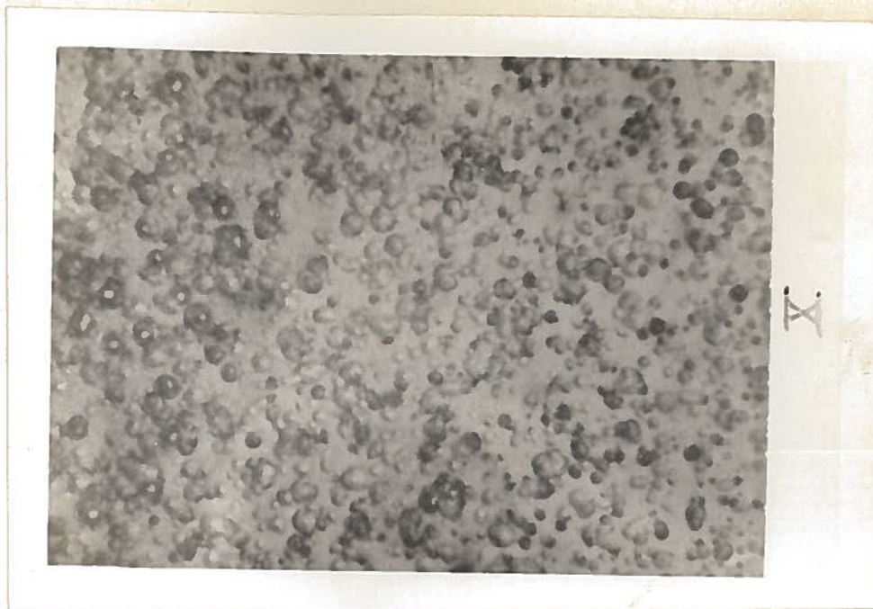
Figure X. Photograph of Cellulose Nitrate Film Exposed to a Fast Neutron Flux Shown in the Uranium Foil-Film Interface
