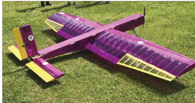
Wing airfoil: Wortmann FX 63-137
