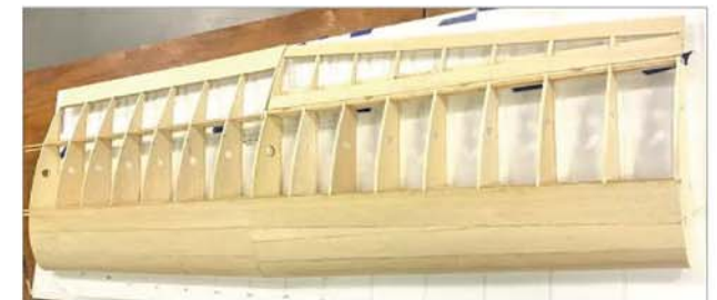
Uncovered 1 st iteration Left Wing and Aileron
