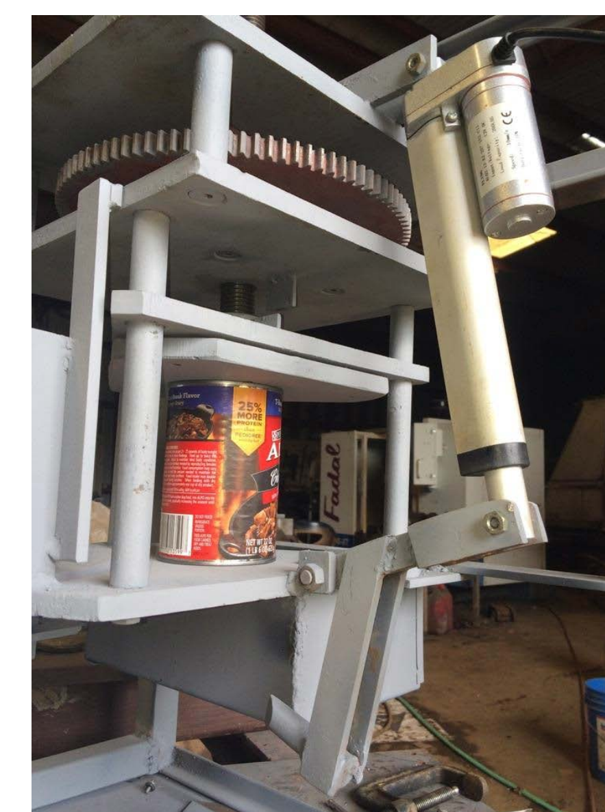
Figure 4: Crushing and Puncturing Mechanism
