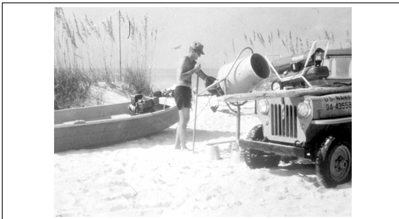
Figure 6. Norwood Rector dyeing sand for a sediment tracer experiment on Fort Walton Beach, Florida.
