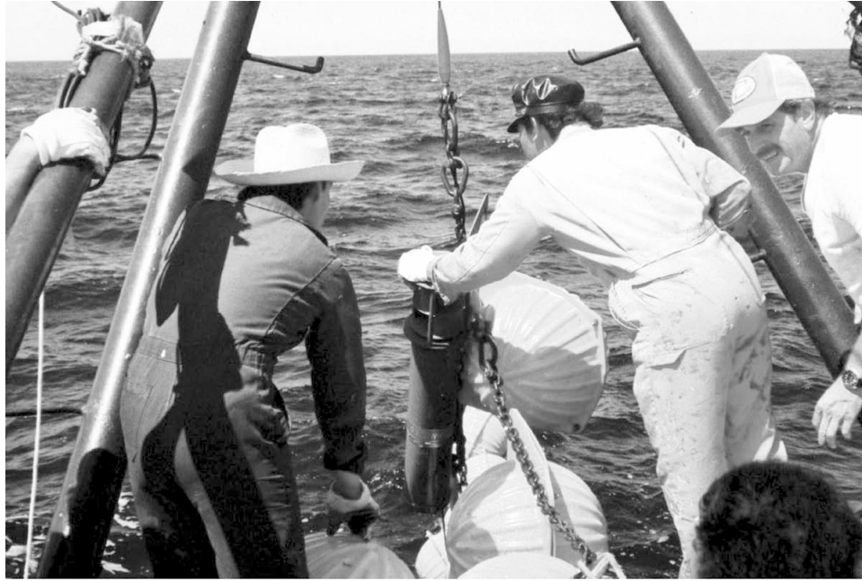
Figure 9. Rod Fredericks is directing the deployment of current meters in the Lombok Strait, Indonesia.
