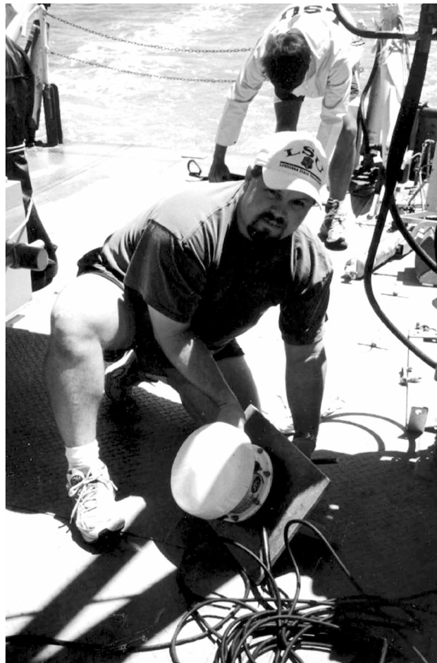
Figure 10. Steve Dartez preparing an ADCP current meter for deployment on a physical oceanography cruise in the Gulf of Mexico.
