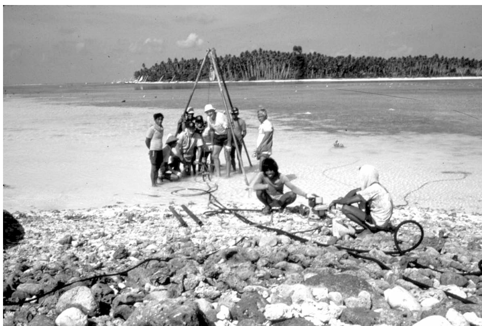
Figure 8. Coring an exposed reef on Toga Toga, a small island along the Sunda shelf margin in Indonesia. Drs. Harry Roberts and Charles Phipps were directing this operations.
